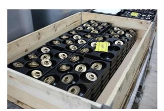
Drives with optimum properties require special designs, meaning a high level of inhouse production. Pictured here are brass gears for worm gears.
