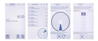
Easy to use: After the desired transaction has been selected, the drum position is shown. After turning the drum by hand, the compartment is marked with a blue light bar and can be opened. Finally, the transaction must be acknowledged.
